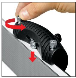
The use of the sidewall planer is essential to remove excess of material which may compromise the file cutting and make it difficult to obtain the right angle.
